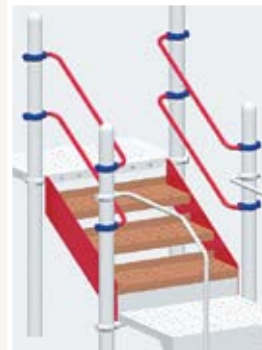
1696-32-81 Stairs with Handrails, 8" (21cm) Riser
