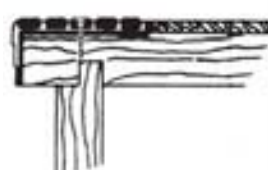
Type 142 Supergrit® attached to wood tread and backed with tile, carpet, or other material.
