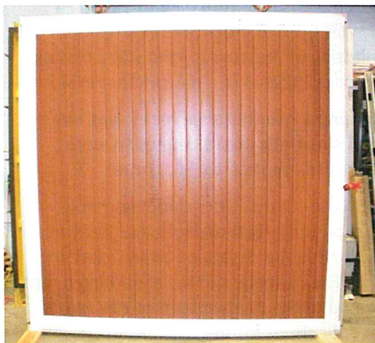
Figure 1: Photos of cladding deflection test specimen showing exterior (left) and interior (right)
