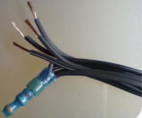
1. Align cables for +/-
