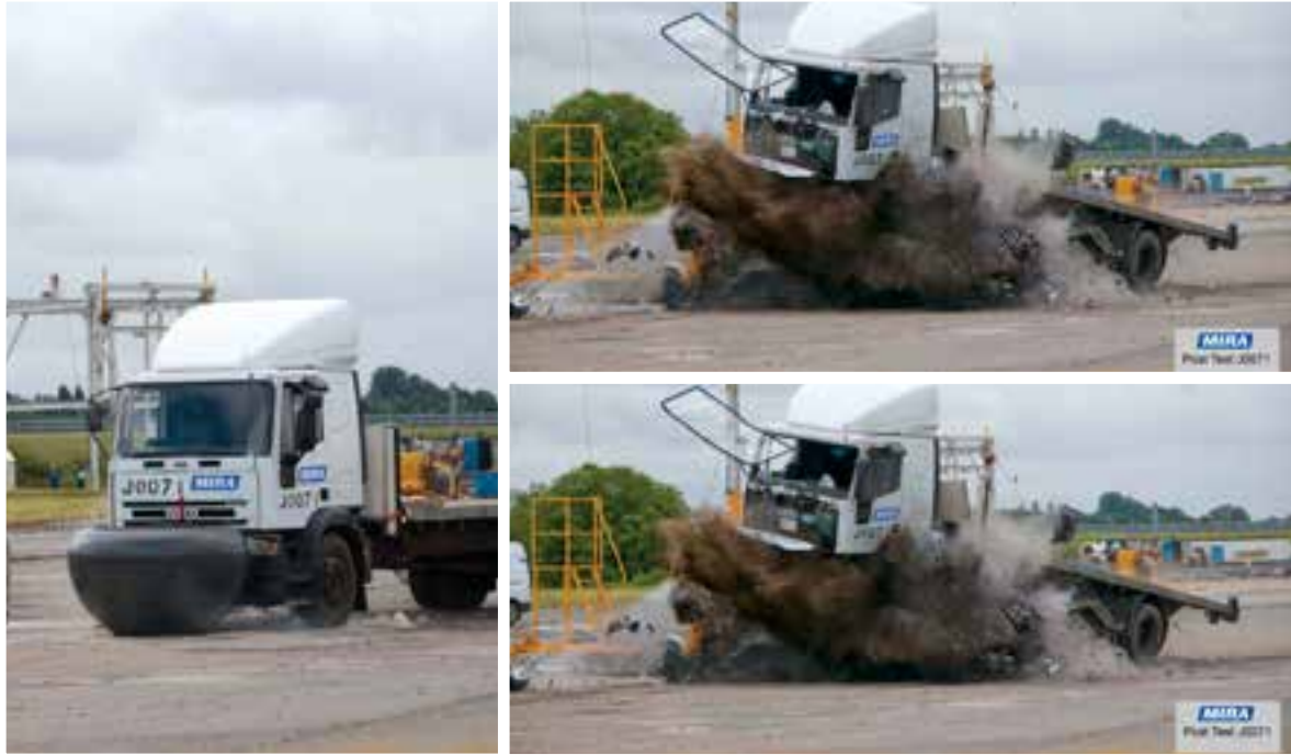
RhinoGuard® Glove Planter crash test
