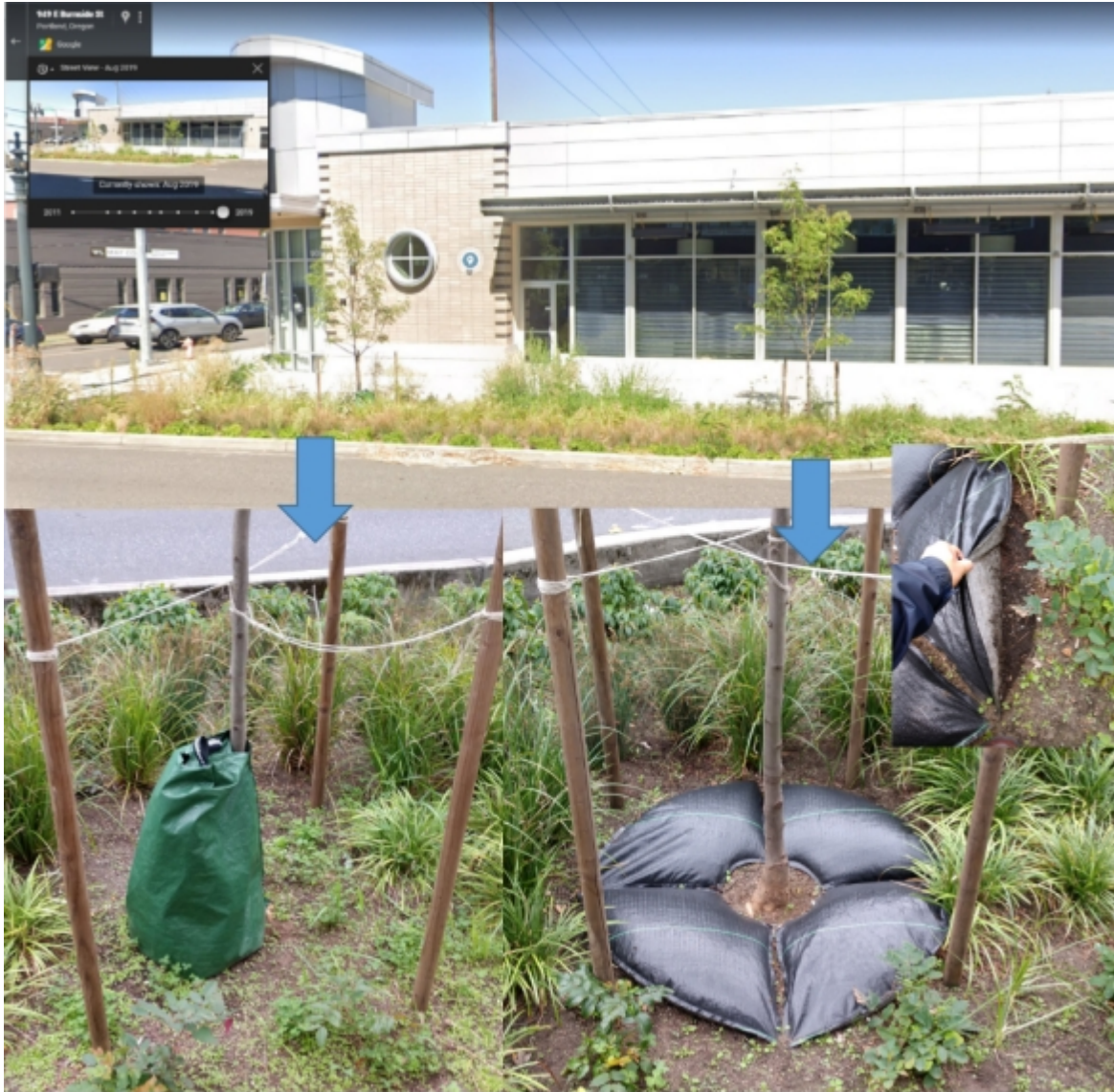
Figure 5. Preliminary trial in Portland OR. Google Street View image (upper) showing two newly planted trees in a roadside GSI. The left side tree was installed with a watering bag that was refilled twice every 17 days. The right side tree has a SWAP system installed.
