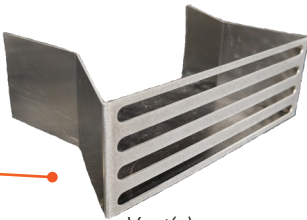
Vent(s) (Vents replace one block and provide support for the next course of block)
