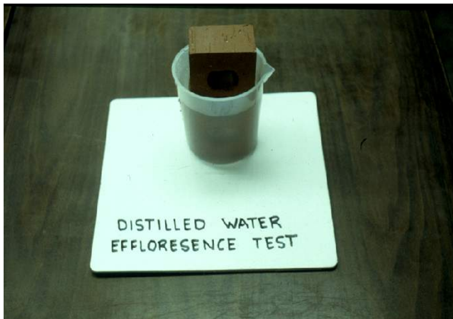
Picture: ASTM C67 Efflorescence Test
