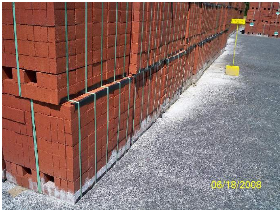
Picture: Salts Migrating Up Cube from Contaminated Base
